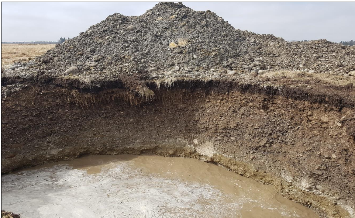
Photograph No. 4: Photograph showing subgrade conditions in Test Pit TP109 at the time of excavation. Photograph taken on 19 th April, 2017.
