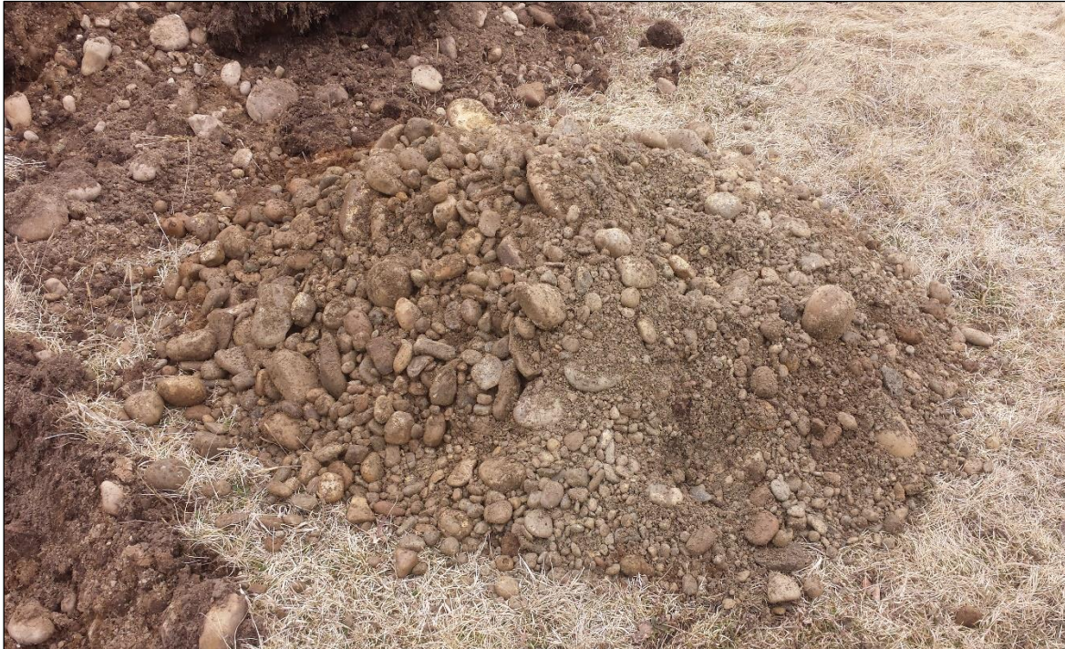
Photograph No. 3: Photograph showing excavated material from Test Pit TP104. Photograph taken on 19 th April, 2017.
