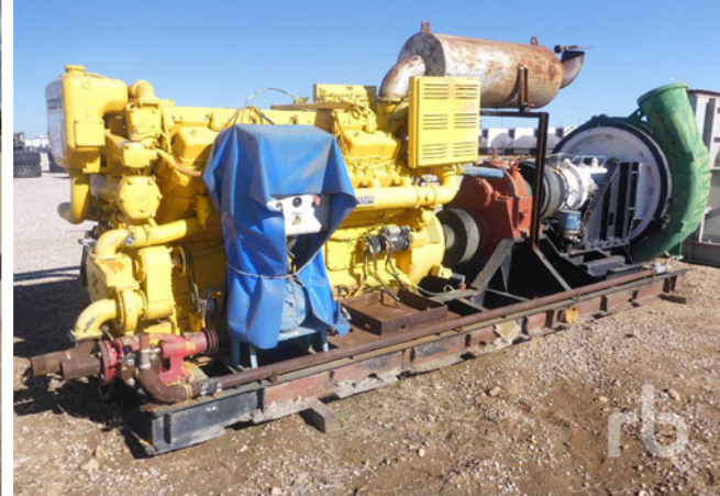
BOOSTER PUMP W-CATERPILLAR V6, 850CV
