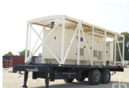
FG WILSON P550E3 550 KVA Skid Mounted
