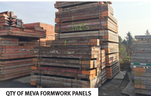
QTY OF MEVA FORMWORK PANELS
