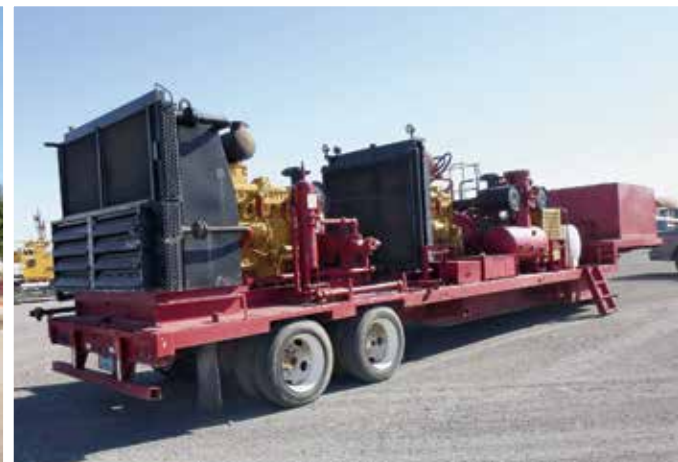
Acid Fracturing Unit
