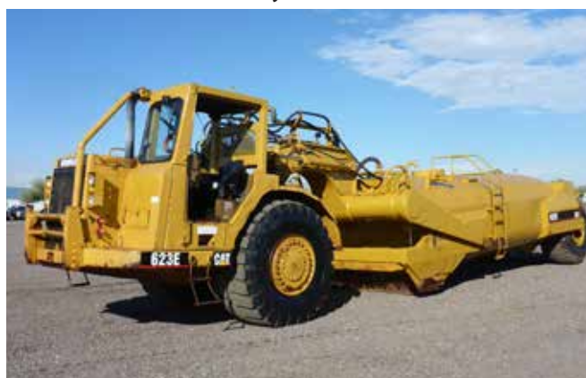
Caterpillar 623E 8000 Gallon Drop Tank
