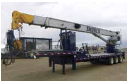
QMC 6082TD 50000 Lb Hydraulic Crane
