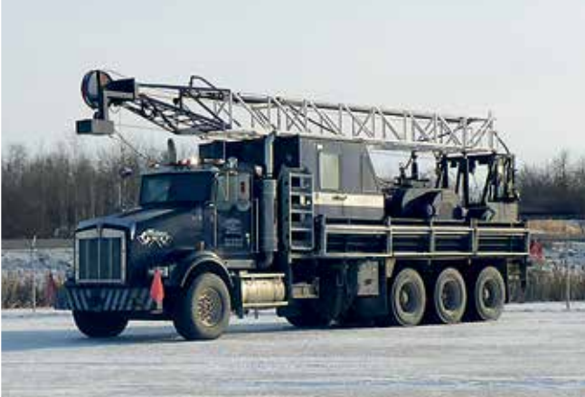
KSM w/Kenworth T800 Swab Rig Well Service Unit
