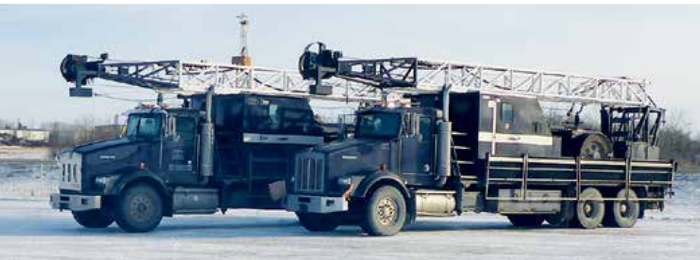
2 – Irontec w/Kenworth T800 Swab Rig Well Service Unit
