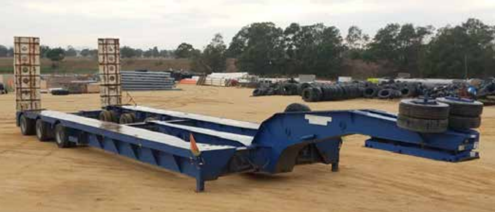
Drake 3 Row of 8 Hyd Widening | Geelong
