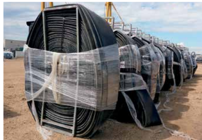
4 – Unused – 200 PSI 12 In. Lay Flat Hose
