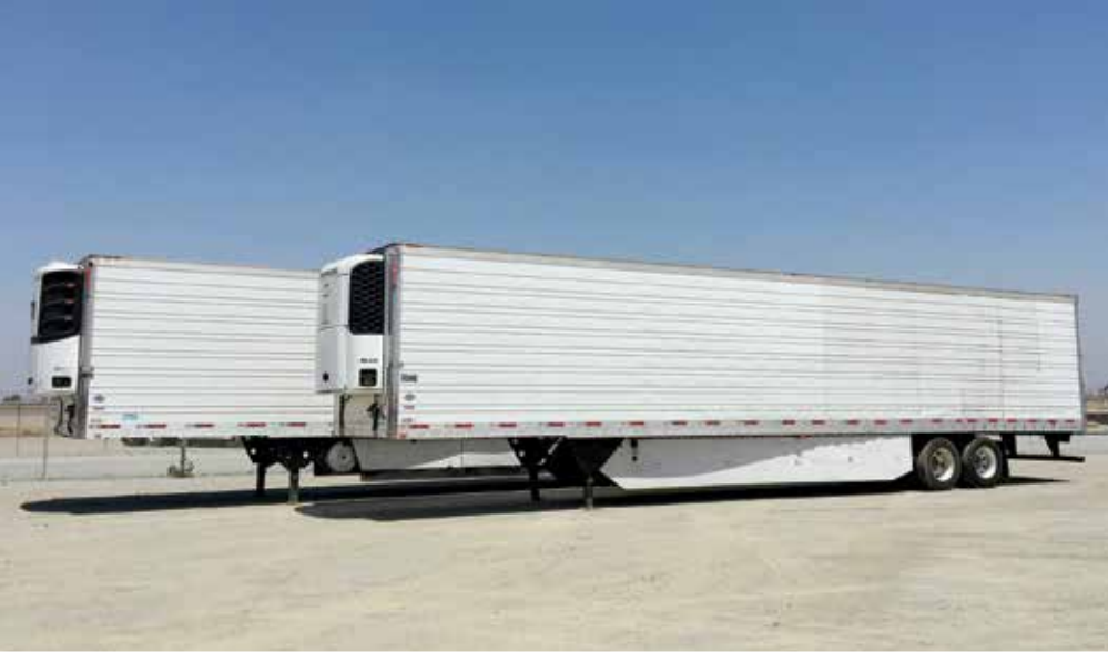
2014 Utility 53 Ft w/2013 Thermo King Precedent S600 & 2014 Utility 53 Ft w/2012 Thermo King SB230
