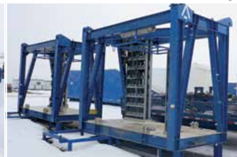
2 – NOV Drill Rig Umbilical Cord Systems
