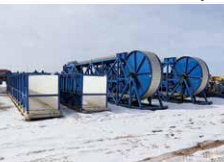
2 – NOV Drill Rig Umbilical Cord Systems
