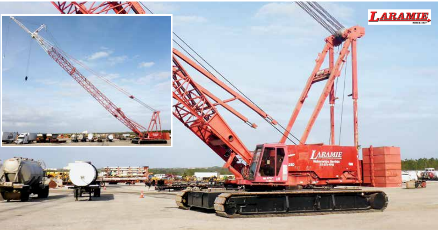
1 of 2 – Manitowoc 2250 300 Ton
