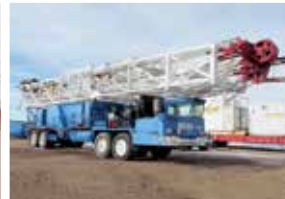
Franks 1287/160 Well Service Rig
